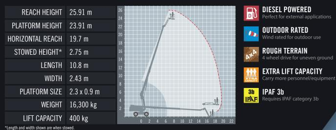
The Manitou 260TJ telescopic boom has a platform with large dimensions that can hold up to 3 operators or 400 kg. The operator is afforded a large working area due to Its rotating pendular arm (+/-70°), and continuous turret rotation capacity of 360° providing flexibility of use.
